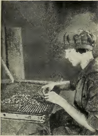
EACH BOLT SLIPS INTO A HOLE To facilitate painting the heads of small bolts, one factory uses this perforated rack. See page 123 for item
